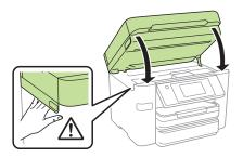
7 If prompted, follow the instructions on the LCD screen. The printer starts charging the ink. Ink charging takes approximately 5 minutes. When you see a completion message on the printer's LCD screen, charging is complete.
