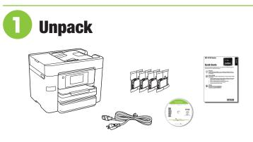
**Note:** Do not open the ink cartridge packages until you are ready to install the ink. Cartridges are vacuum packed to maintain reliability.
